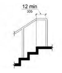
FIGURE 11B-505.10.2 TOP HANDRAIL EXTENSION AT STAIRS
