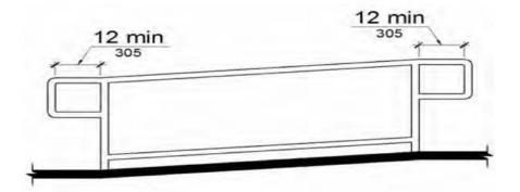
FIGURE *11B-*505.10.1 TOP AND BOTTOM HANDRAIL EXTENSION AT RAMPS
