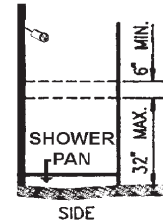
(c) LOCATION OF GRAB BAR REINFORCEMENT FOR ADAPTABLE SHOWERS
