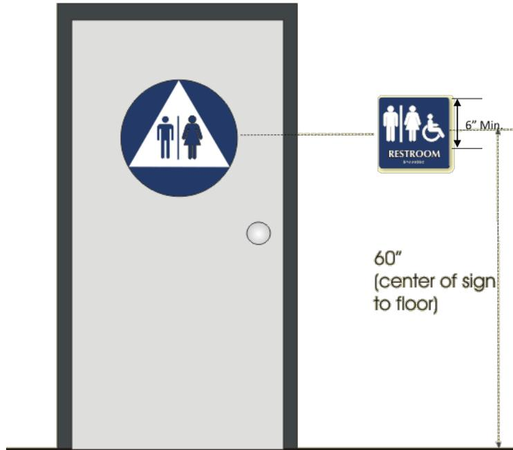
**11B-703.6.1 Pictogram Field.** Pictograms shall have a field height of 6 inches (150 mm) minimum. Characters and braille shall not be located in the pictogram field.
